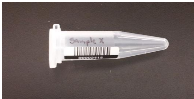
Figure 1. Necessary barcode label placement on a 1.7 mL microcentrifuge tube containing sample DNA.
