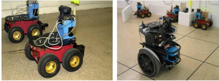
Fig. 10. The Robot Hardware: Pioneer 2AT and Segway RMP.
