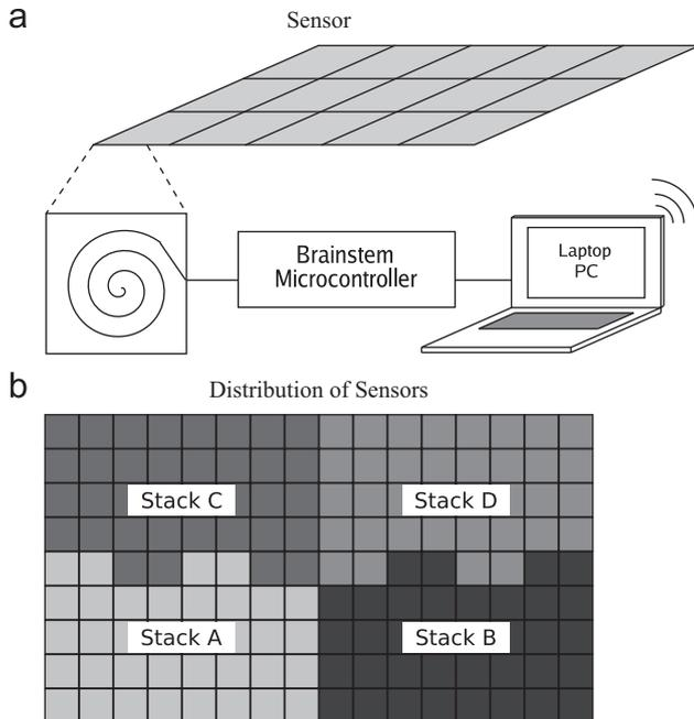
Fig. 11. Sensor layout in the laboratory environment: (a) sensor and (b) distribution of sensors.
